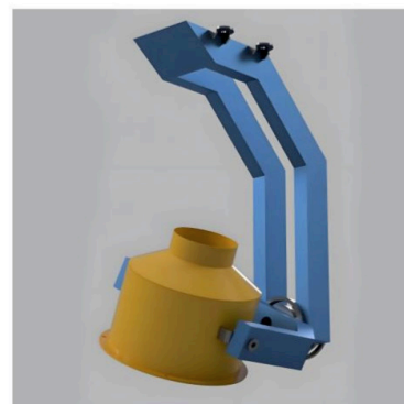
UNIDIRECTIONAL COOLING AIR VENT MODELING
